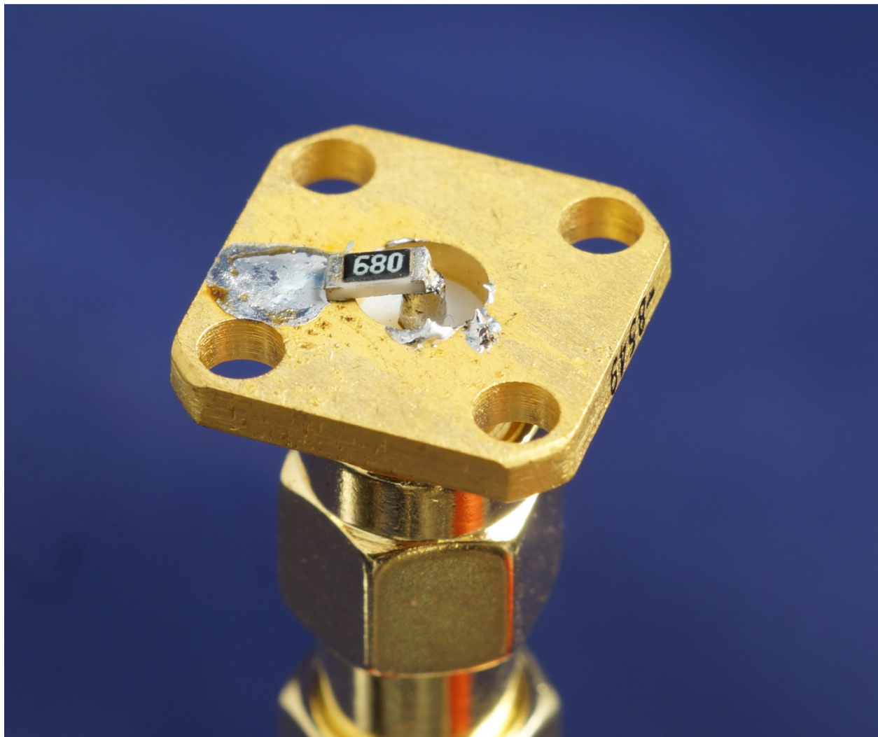
Figure 8 – Simple 68-ohm coaxial termination
