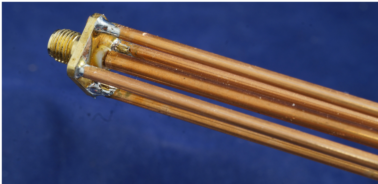
Figure 1 – Open coaxial line made from hobby tubing
