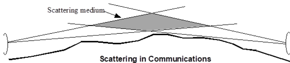
Figure 1. Over-the-horizon contacts made by radio amateurs usually involve scattering.
