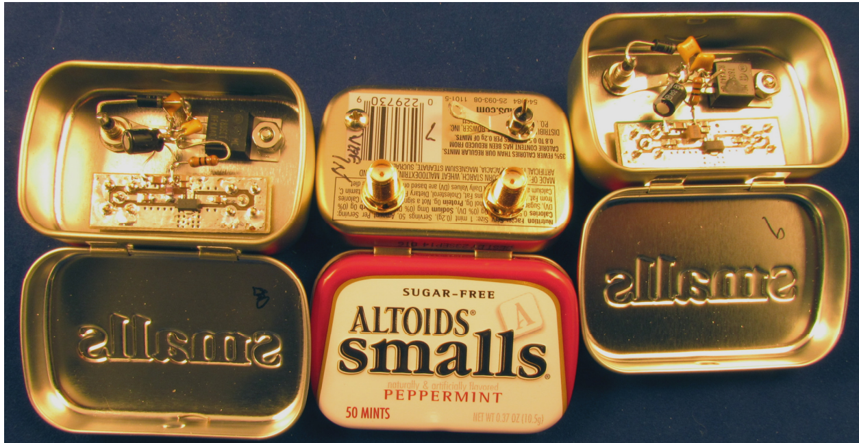
Figure 5 - MMIC preamps in small Altoids tin
