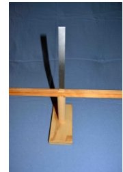
Knife-edge diffraction set-up
