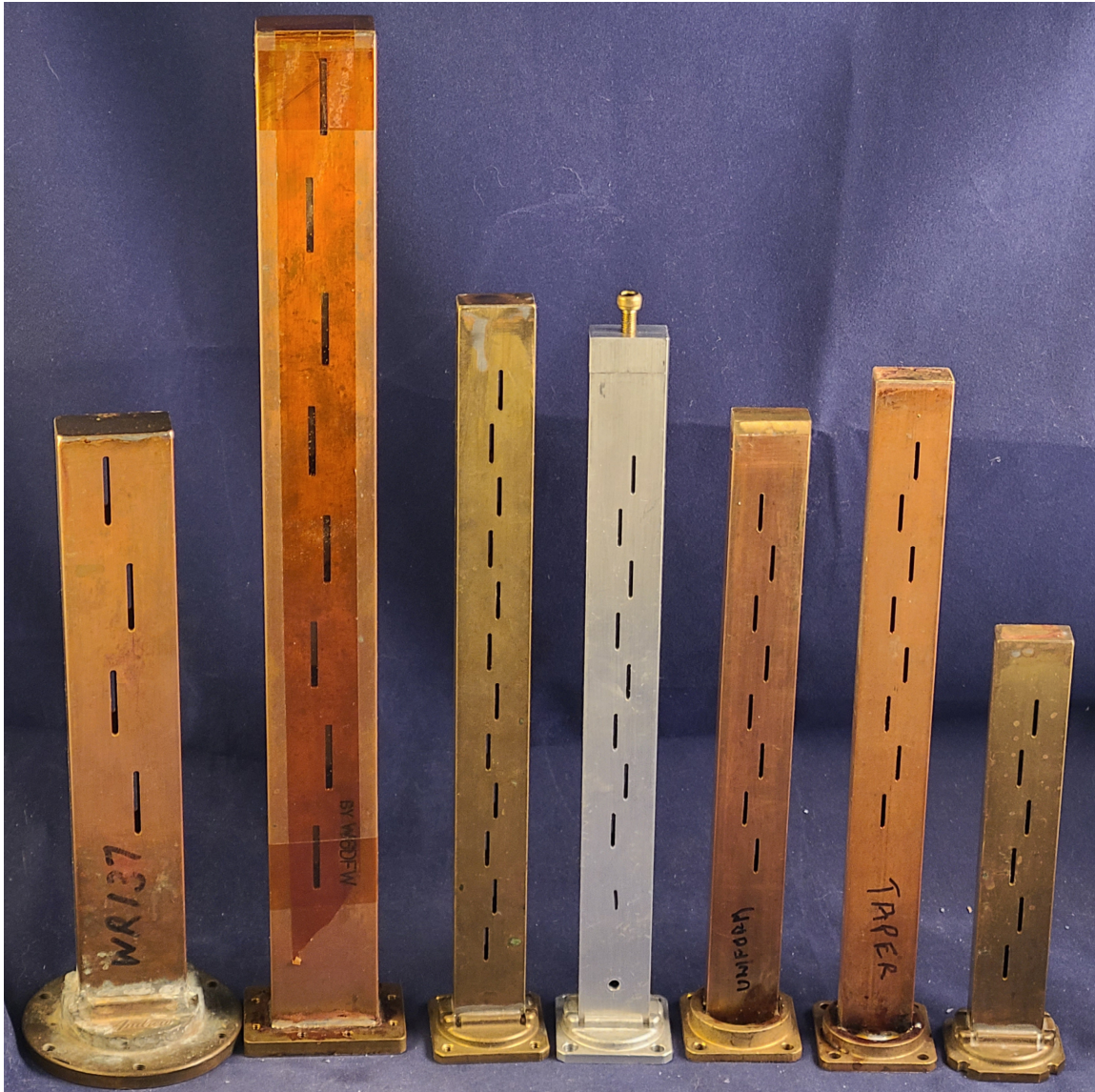
Figure 3 – Waveguide Slot Antennas, from Left to Right:
