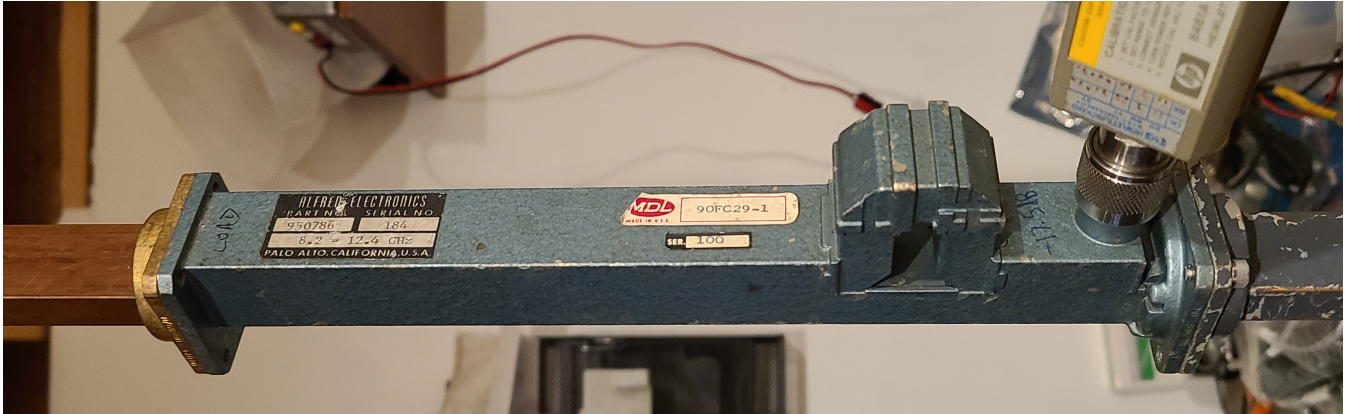
Figure 18 – Alfred Electronics X-band directional coupler with high directivity
