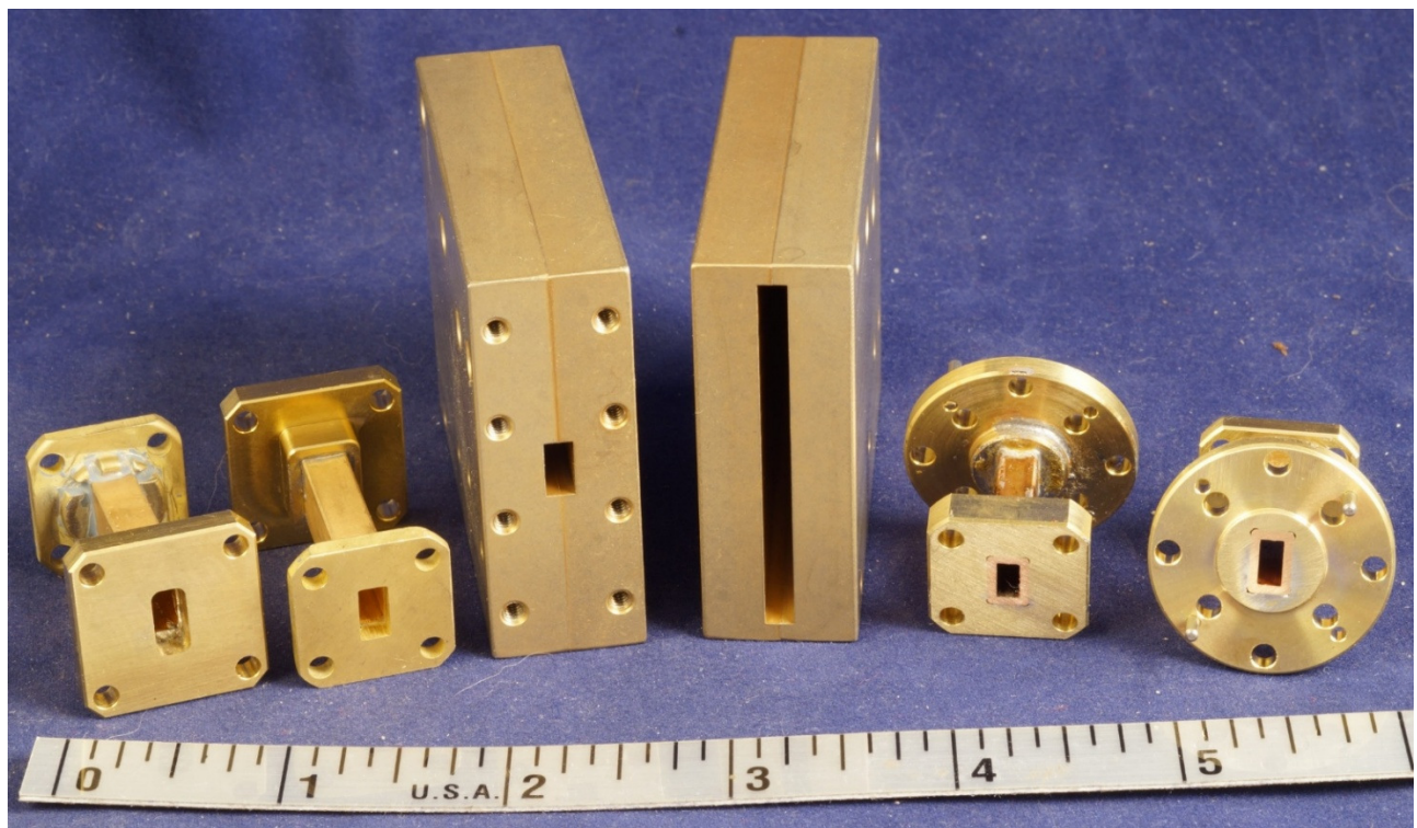
Figure 17. W1GHZ Sector horn, back and front, surrounded by WG adapters for WR42 and WR22/19
