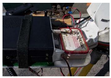
Figure 3 The Dash-Sender in the Altoids box keying my FT-817 in the 10 GHz contest 2006.
