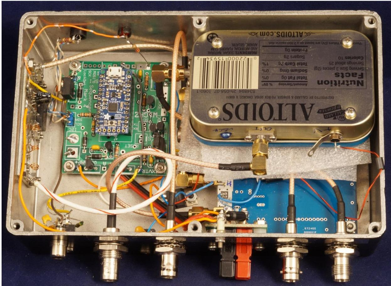
**Figure 6 – Complete modernized 432-MHz transverter with lid removed**
