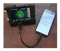
To continue setting up TCPUART, make sure the baud rate is 115200 and press 'Connect'. The label will change to 'Disconnect' which actually means you are connected. Your Cell Phone will likely ask you if you want to give TCPUART the right to rummage around in your phone so it can find a device. Answer 'OK'.
