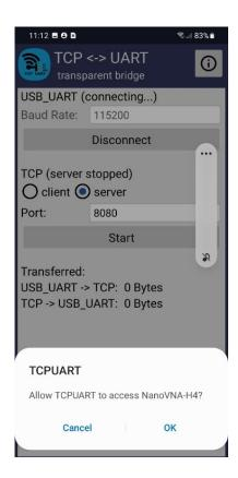
Next, for the TCP part, select 'Server' and check that the port is set to 8080 then press 'Start'. The label will change to 'Stop' which means you are connected.
